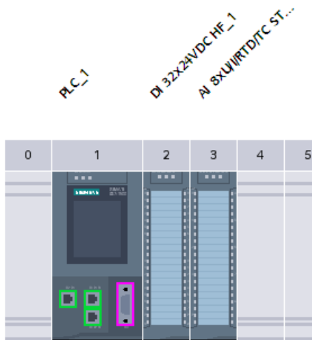
Figure 7-4 Result of the hardware detection in the device view
