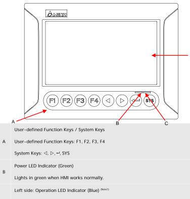
С The operation LED indicator blinks in blue when either the communication is carried
