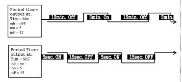
\* Period Timer will operate being isolated from the operation of Thermometer.
