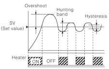
As like above picture, the control value is up and down by set value, it is called Hunting. And Overshoot is occurred at initial point when just power on. If the Hunting and Overshoot is less, it will be a good control.
