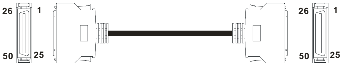
Figure 15 UC-ET010-15B (1 m) Female MDR50 connector ↔ Female MDR50 connector
