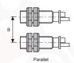
When sensors are mounted on metallic panel, you must prevent the sensors from malfunction by any metallic object. Therefore, be sure to keep a minimum distance as below charts.
